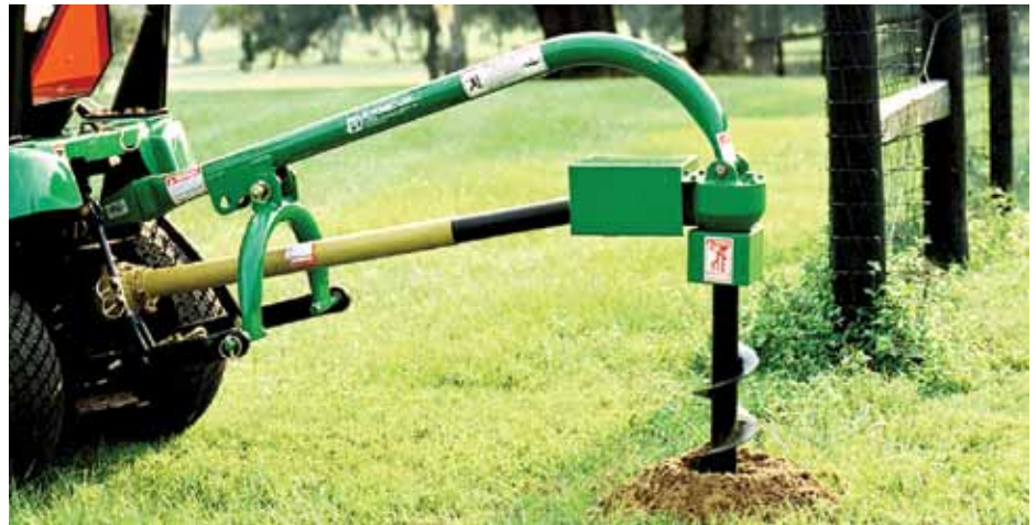
Check for utility lines before digging to prevent damage, especially when the task calls for a deeper hole, such as one requiring the use of a post hole digger.
